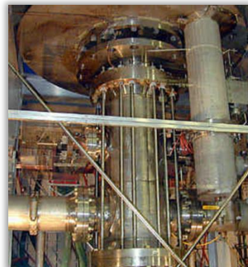
NHMFL 45T coil insulated with CTD-101K
